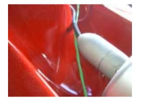
162. Make a mark on the fuselage in front of your starter motor.
