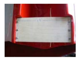
158. Measure the distance between the mounting holes on your turbine mounting bracket. Make allowances for the mounting screws.
