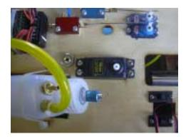
144. Install your receiver as shown, using a tie wrap.
