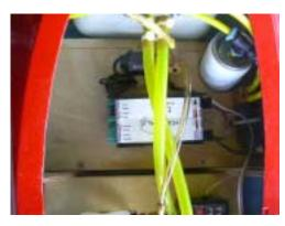
180. Secure the fuel pump up forward as shown. You want the pump away from the receiver and ECU to prevent any possible electronic interference.
