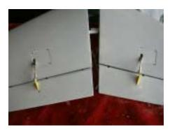
115. All of your servos are installed, now it is time to glue in the horns. Follow the same procedures for all seven horns. First use masking tape to tape the control surfaces to keep them from moving.
