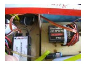
194. Plug in your ECU battery and stuff it in the nose. Do not secure it yet. You need to move the ECU and radio battery packs to achieve final balance. When balance is properly achieved, the batteries can be mounted into place with silicone glue or heavy duty Velcro. Make them very secure.
