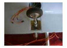
122. Use masking tape to hold the horn and linkage at 90' to the surface while drying.
