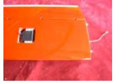
105. Drill pilot holes in the wooden mounts and secure the servo with the kit-provided screws. Do not over tighten and strip the screw holes.
