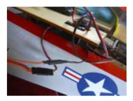
148. Run these extensions through the holes in the nose gear formers, up into the extreme nose area.
