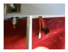
127. Using the one of the two longer silver bolts, plus a washer, provided in the kit, secure the elevator assembly to the right-hand boom. Tuck the servo cable and connector into the elevator assembly. Do not over tighten this bolt, and be careful with the stab and single boom assembly while it is being assembled, it is easy to damage before it is added to the fuselage and the second boom joined for support.
