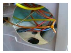
189. Connect the propane line from the engine to the propane solenoid, through the hole in the bulkhead shown.
