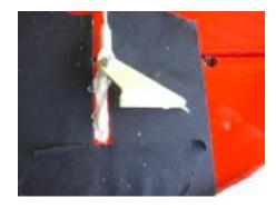
119. Insert the control horn into the slot, making sure it is 90' to the surface, and not too deep and not too shallow in the slot.
