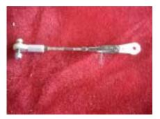
82. Attach the horn and linkage to your servo.
