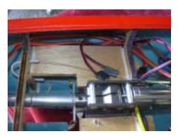
150. Check all your wiring and plumbing beneath the radio tray, then secure the tray with the provided two screws. Note how the airlines go around the side of the tray and over to the bottom. Be extra careful about pinching or kinking airlines.
