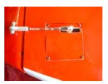
87. Prepare all the control horns. Roughen up the bottom portion on both sides using 40 grit sandpaper, to give a better gluing bond.
