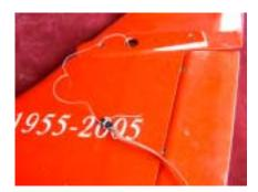
97. Fair the extension into the string with masking tape as shown to keep the connector from snagging on the internal structure.
