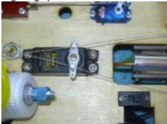
152. Lower the gear. Pull the steering wires taut, while sighting through the nose gear opening in the fuse to keep the nose gear straight, and tighten the EZ connectors. You only need the steering wires free of slack, not tight. If they are overly tight, they may keep the gear from locking down.
