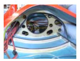
139. Slide the tank into place. Make sure it is square and butted against the former behind it. Use some silicone glue for extra security. Silicone keeps the tank in place, but still leaves it easy to remove in case service is needed.
