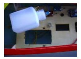
141. Install the UAT using a tie wrap. Note most UAT devices need to be installed at angle. Follow the manufacturer's instructions. Also note that some UATs may project high enough that you will either need to make a hole in the plastic cockpit deck or relocate the UAT, or simply not use the cockpit deck.
