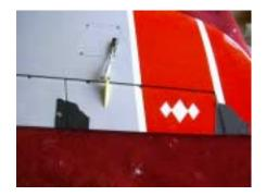
116. Surround each control horn slot with masking tape, leaving a 1/8" border all around. Do not tape the area in front of the horn, only the two sides and the rear.
