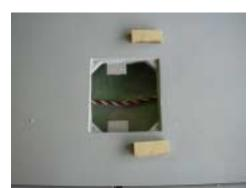
110. Epoxy those blocks into place, level with the existing mounts. Do not epoxy them to the mounts, but only to the wings and to the little corner triangular blocks that hold the servo cover hold-down screws.
