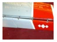
8. Carefully align the trailing edges of the flap and aileron surfaces, using the trailing edge of the wing at the tip, and the paint stripes, as a guide.
