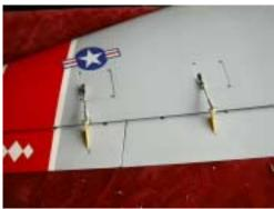
109. Install the flap servo into the right wing normally. For the left wing, do this: Cut two scrap plywood blocks as shown, the same width as the existing servo mounts, but about 1" long.
