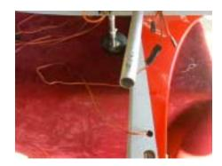
129. Slide the boom into place. Make sure the two remaining extensions from the fuselage go out through the holes in the boom to where the wing will be, and make sure you do not pinch the airlines for the retract mechanism.
