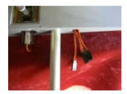
126. Plug the elevator servo into the extension in the right side boom. Secure the connection with masking tape.
