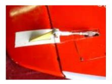
94. You will need to feed a heavy-duty 22-gauge 36-inch extension through the right side boom for the elevator servo. Feeding extensions through the structure can either be a very tedious, time-consuming, and frustrating process, or you can follow my technique and it will only take a minute. All you need is a weight such as a wheel collar, a little bit of string such as dental floss, and a little bit of masking tape. Tie the wheel collar to the string, and read on.
